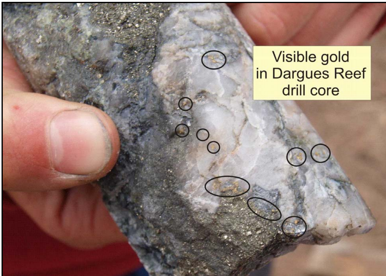
Figure 2: Coarse gold in quartz veining within a broader sulfide lode. Results pending.
