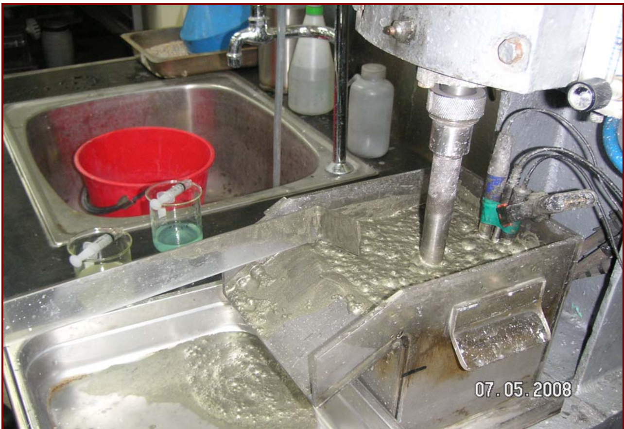
Figure 1: Sulphide concentrate being 'floated' during laboratory test work on Dargues Reef mineralised material.
